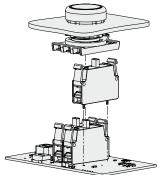
A number of new EROUND contact blocks provided with pins to be welded are now available. These contact blocks, available in panel-mounted versions, are suitable in cases where a printed circuit is used instead of wiring, and therefore the contact blocks are welded directly onto the printed circuit.
