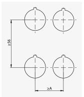
Fixing adapter with 3 positions A=30 mm
