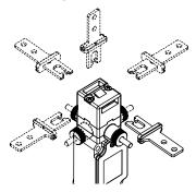
The head can be quickly rotated on each of the 4 sides of the switch by unfastening the two fixing screws. The mechanical delay device can be rotated in 90° steps as well. This enables the switch assume 32 different to configurations.
